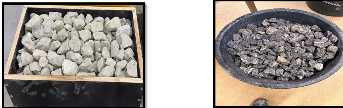
Figure 6 Not washed Ballast (Left) and washed ballast (Right)
