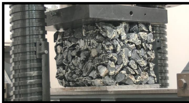
Figure 7: Sample of class IV being tested in compression.
