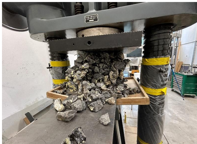
Figure 11 Sample 1_10: Even compression plate with visible ballast separation at the bottom, indicating adhesive concentration gradient
