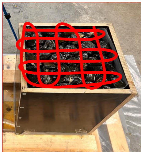
Figure 3 : Gravitational application of the ballast bonding resin (mesh path)
