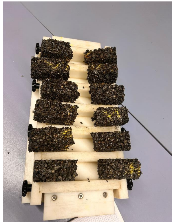
Figure 16 : 3-points bending test on small samples
