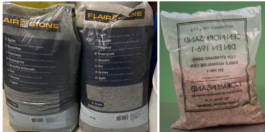
Figure 14 : Crushed aggregates 1-3 and 2-5 mm (left) – Normensand (right)
