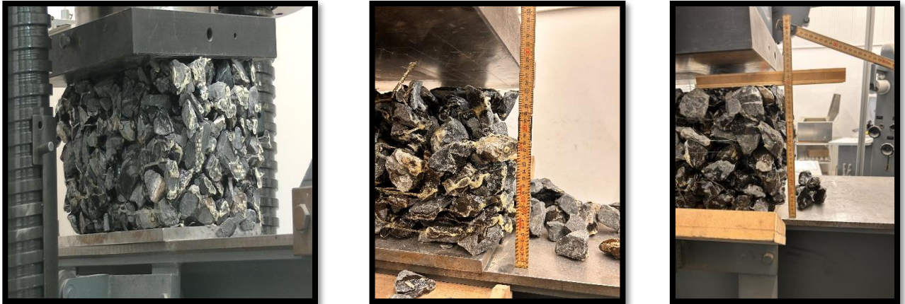
Figure 10 Sample 1_8 during and after compression testing: Left - Uneven compression observed; Middle - Bottom side at 26 cm post-test; Right - Top side at 29 cm post-test, illustrating the gradient in adhesive distribution and its impact on sample integrity
