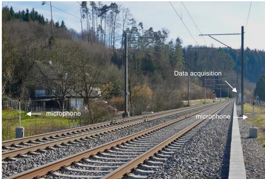
Figure 1: Photo of a noise monitoring station on the line between the cities of Zürich and Winterthur in Switzerland. Photo credit: own work by the author.
