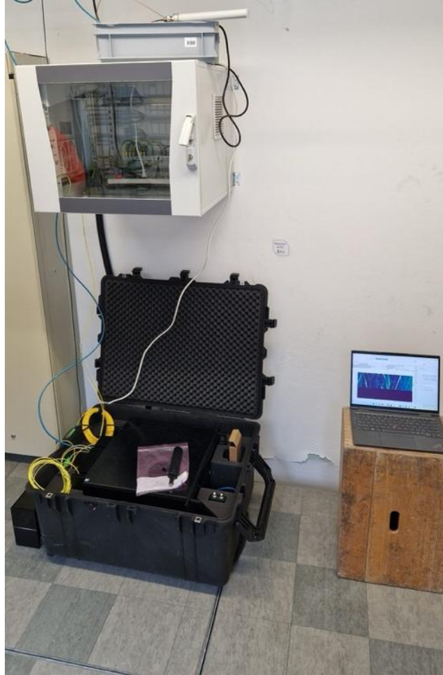
Figure 2: DAS deployment in the telecommunications facility at Vernayaz. The Sintela Onyx interrogator was connected to 2 existing railway telecommunications fibers and operated directly from its transport case. System configuration and remote access were provided through a laptop and an independent 4G router. The setup doesn't require much space and can be deployed rapidly within existing railway infrastructure facilities.
